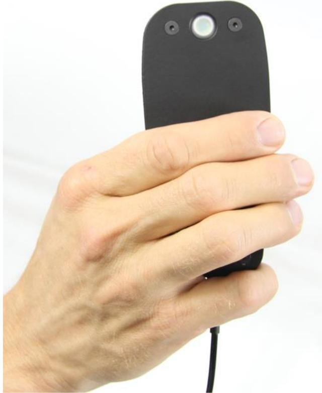
To make a measurement press the Start/Pause button and move the the LabFlicker towards the lamp you want to measure, with the sensor facing the lamp.
