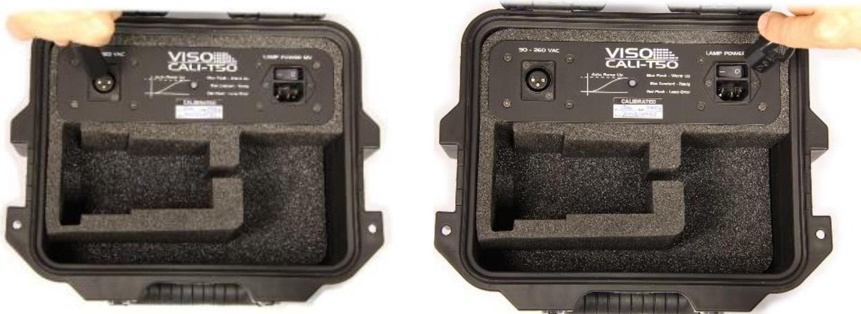
The lamp needs to ramp up, and there is an indicator with a mini instruction on the box. The blue flashing indicator means the lamp is ramping up, a constant blue colour defines the lamp is ramped up, whereas the red colour of the indicator means there is an error.
