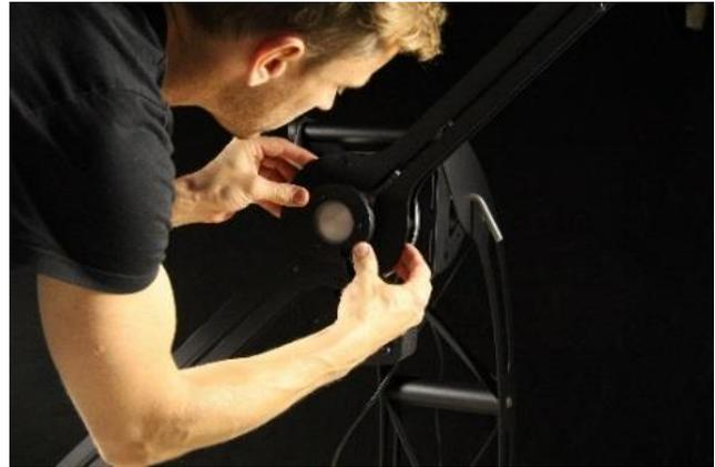
Then place the sensor approximately two meters away (*recommended to use approximate same distance as defined on certificate*) from the setup with the reference lamp. Make sure the sensor is aligned with the lamp. Shoot the laser towards the lamp glass and catch the reflected beam in the same area of its origin, or within a 4 cm area. Such a procedure puts both the sensor and the lamp in alignment. The pictures below explain the process:
