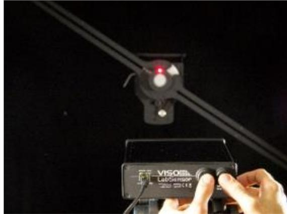
The glass surface of the lamp produces a lot of internal reflections of the laser beam, and it complicates the exact distance calculation. The precise distance determination is essential in achieving the best results. That is why a fixed white target point was designed above the lamp luminous area.
