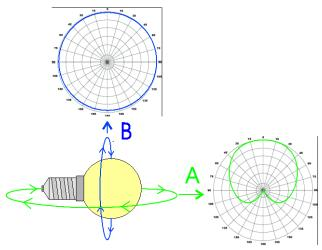
The principle behind it is based on a consideration that the opposite field "B" is circular (see in the picture above). Most of the light sources and fixtures have nonuniform circular "A" and "B" fields. In some particular cases the deviation from a circular uniformity of the "B" field is caused by a physical geometry of the light source. A series of test measurements of different types of light sources was made to account for such errors.
