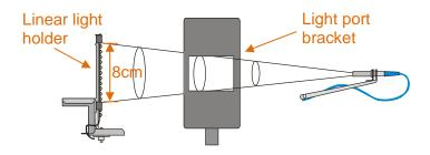
The "light port bracket" ensures that only 8cm of the linear light source is captured. The actual length of the light source is then inserted into the software after the measuring process is finished.
