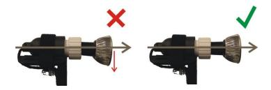
After alignment turn the light source back pointing straight towards the optical sensor.
