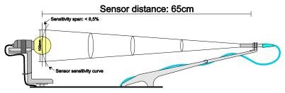
The system is constructed for measuring light sources with a maximum diameter of 100mm. It is calibrated with the help of a calibration source with an aperture diameter of 35mm with
