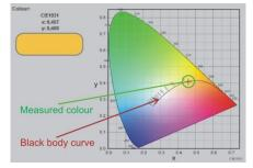
corresponding to the measured colour is shown with a black cross. It can be used to check the whiteness of a colour, by checking how close it is to the black body curve: the closer it is to the black body curve the more accurate is the white colour.
