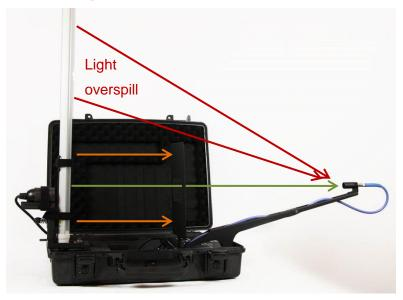
Light overspill, which is the light received by the detector outside of the light port bracket area, can increase the measured value of the luminous flux.
