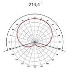
The complete 360 degrees angular light field is then measured and the beam angle is calculated.
