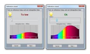
6. Click next and cover the sensor or turn off the calibration source so the dark reference spectra can be measured.
