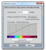
4. Make sure the calibration source has been turned on for some time or at least 30 min so the output is stable.
