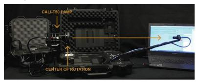
The lamp must be pointed directly towards the sensor. Sometime is might be necessary to unplug RJ45 cable to the motor to enabling precise alignment.
