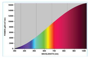
Calibration sources can be obtained from a number of suppliers, in this example will we use the CALI-T50 from Viso Systems which is a tungsten irradiance lamp. The spectrum of the calibration source is usually provided in a .Imp file (lamp file).
