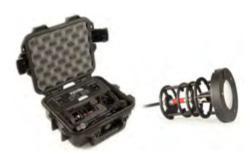
The LabSpion includes a tungsten irradiance reference lamp and auto ramp-up power supply. This reference lamp can be used to verify your calibration at any time without the need for external support. It is easliy mounted in the center bracket of the LabSpion.
