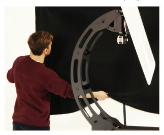
The LabSpionTM uses a directional spectrometer sensor which makes it possible to capture light measurements in room which is not dark. This means that, when you need to make measurements, you can utilize any space at your facility which is available.
