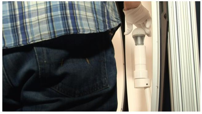
After the light source has been on for 5 min in the integrating sphere the total luminous flux in lumen, color temperature and power are measured.
