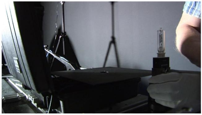
The lumen value is calibrated using an omnidirectional light source with a known lumen value measured by DTU in their integrating sphere.
