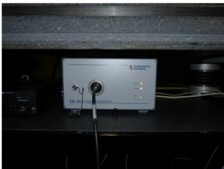
Power source CW1251 Constant voltage and low distortion
