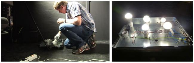
Light sources are monitored for stable light output before the measurement is made.
