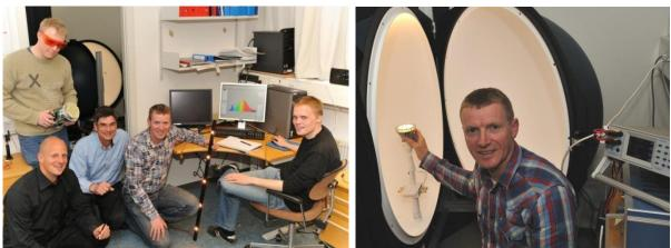
A series of light sources has been chosen for testing accuracy. Initially, the light sources are measured using the integrating sphere of DTU. Then the same light sources are measured using the LightSpion and the two results are compared.
