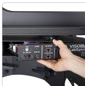
The main board easily slides out allowing a quick update
