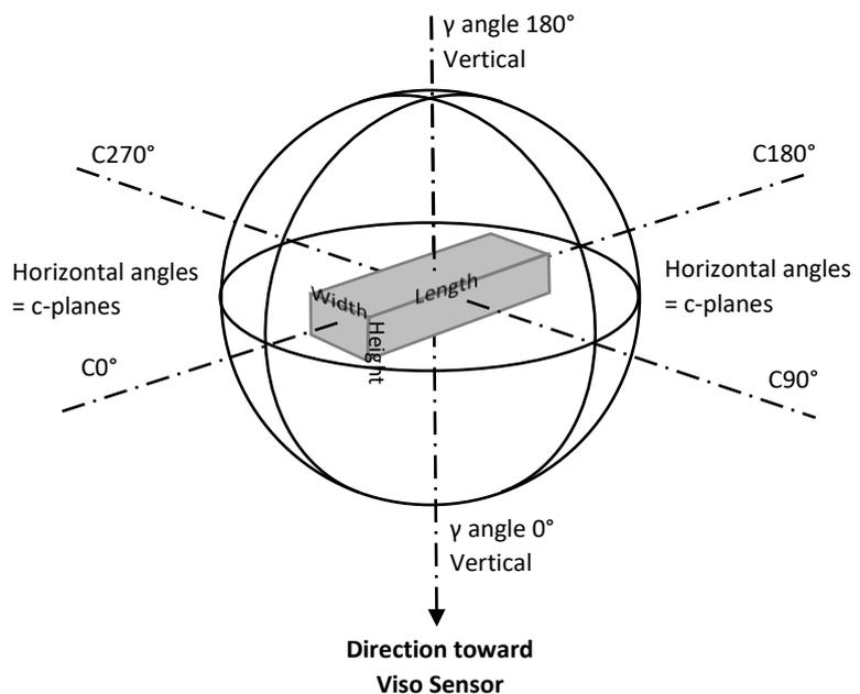
The image to the left shows the C-plane orientations of the LabSpion. BaseSpion and LightSpion work the same way).
