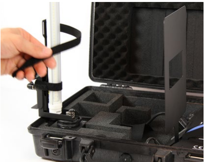
4) Use Velcro straps to hold fixture. Do not cover the middle 8+ cm. This section
